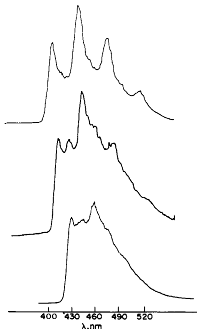
Figure 1. Phosphorescence spectra at 77 K in MCIP glasses of three substituted \alpha -trifluoroacetophenones: top, p -CF 3 ; middle, p -CH 3 ; bottom, p -OCH 3 .
